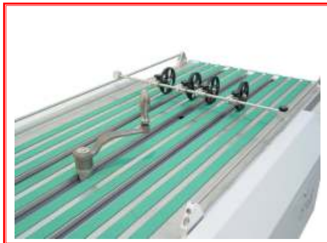
Fig 1.2 Lowering the Feet with the Adjustment Tool
